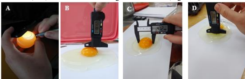
Figure 1. (A) Candling egg; determination of (B) the height and (C) diameter of egg yolk; (D) determination the height of egg white
