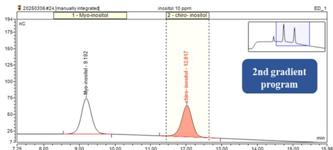
**Figure 2.** Chromatogram of a dietary supplement sample containing myo-inositol and D-chiro-inositol using gradient program 2
