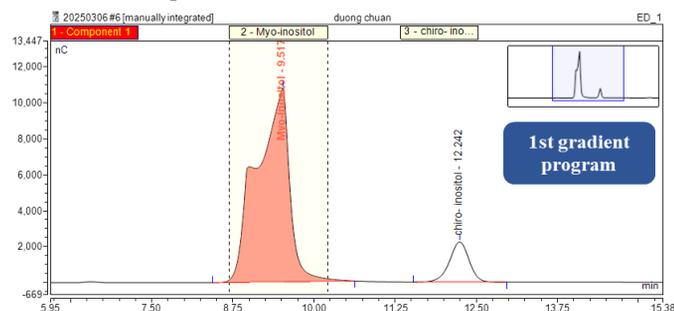
**Figure 1.** Chromatogram of a dietary supplement sample containing *myo*-inositol and *D-chiro*-inositol using gradient program 1
