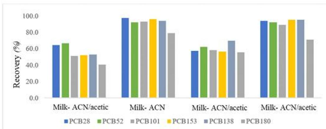
**Figure 2.** The recovery efficiency of 6 I-PCBs in two investigated extraction solvents
