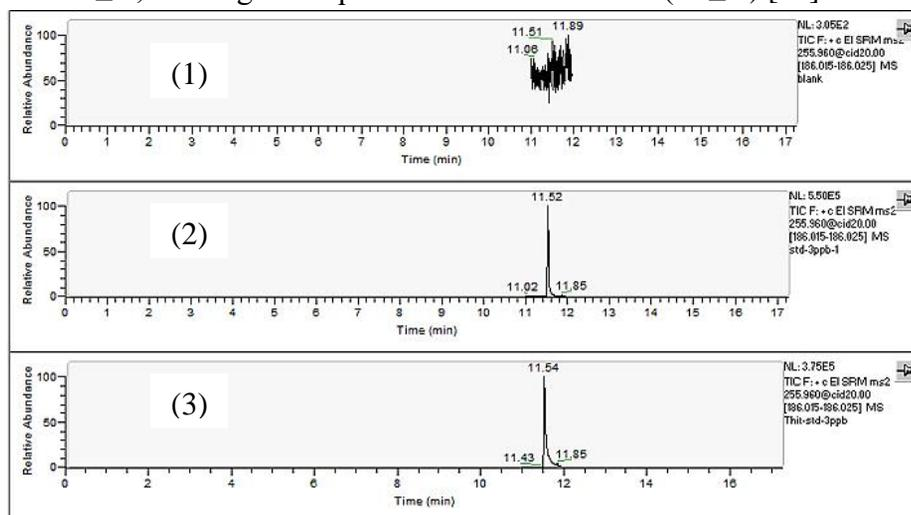
**Figure 6.** Chromatogram assessing the specificity of PCB-28 ((1) Blank sample; (2) Standard sample in solvent; (3) Blank sample spiked with standard)
